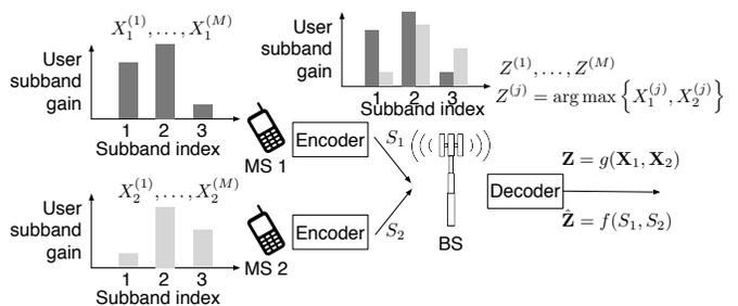
Fig. 1. The BS wishes to compute the index ( $\arg \max$ ) of the user with the largest gain on each subband. The users encode their local gains across subbands using SQs.
