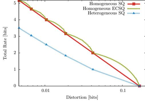
Fig. 4. SQ R-D curve for channel capacity distributed Uniform(0, 1).
