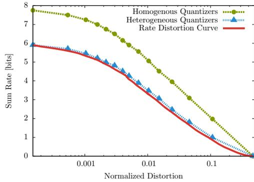
Fig. 6. Comparison of HomSQ and HetSQ to R-D function for a uniform distribution on the LTE defined CQI values. The distortion (average capacity loss) has been normalized by the average channel capacity.
