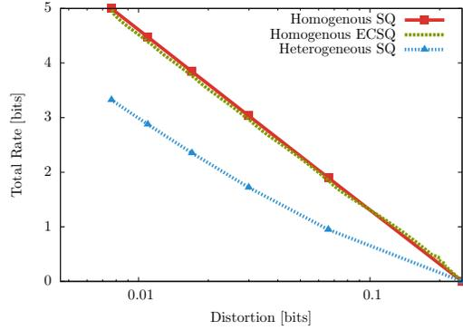
Fig. 5. SQ R-D curve for channel capacity distributed Exponential(2).
